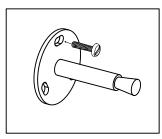
Measure complete slide bar from center of the escutcheon to the center of the other escutcheon. Transfer those dimensions to the mounting surface. Attach mounting brackets to the wall. It is highly recommended that the brackets be mounted into a vertical stud.
