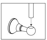
Install slide bar into lower escutcheon. Make sure notch in slide bar fits into the pin in the escutcheon. This will prevent any rotation of the slide bar.
