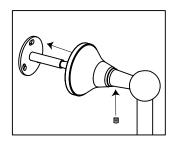
Install slide bar into upper escutcheon and trim ring. Install assembly to the upper mounting bracket. Make sure notch in slide bar fits into the pin in the escutcheon. Tighten set screws securely
