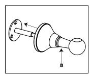
Install escutcheon and trim ring to the lower mounting bracket. Use set screw to tighten escutcheon to post of mounting bracket.
